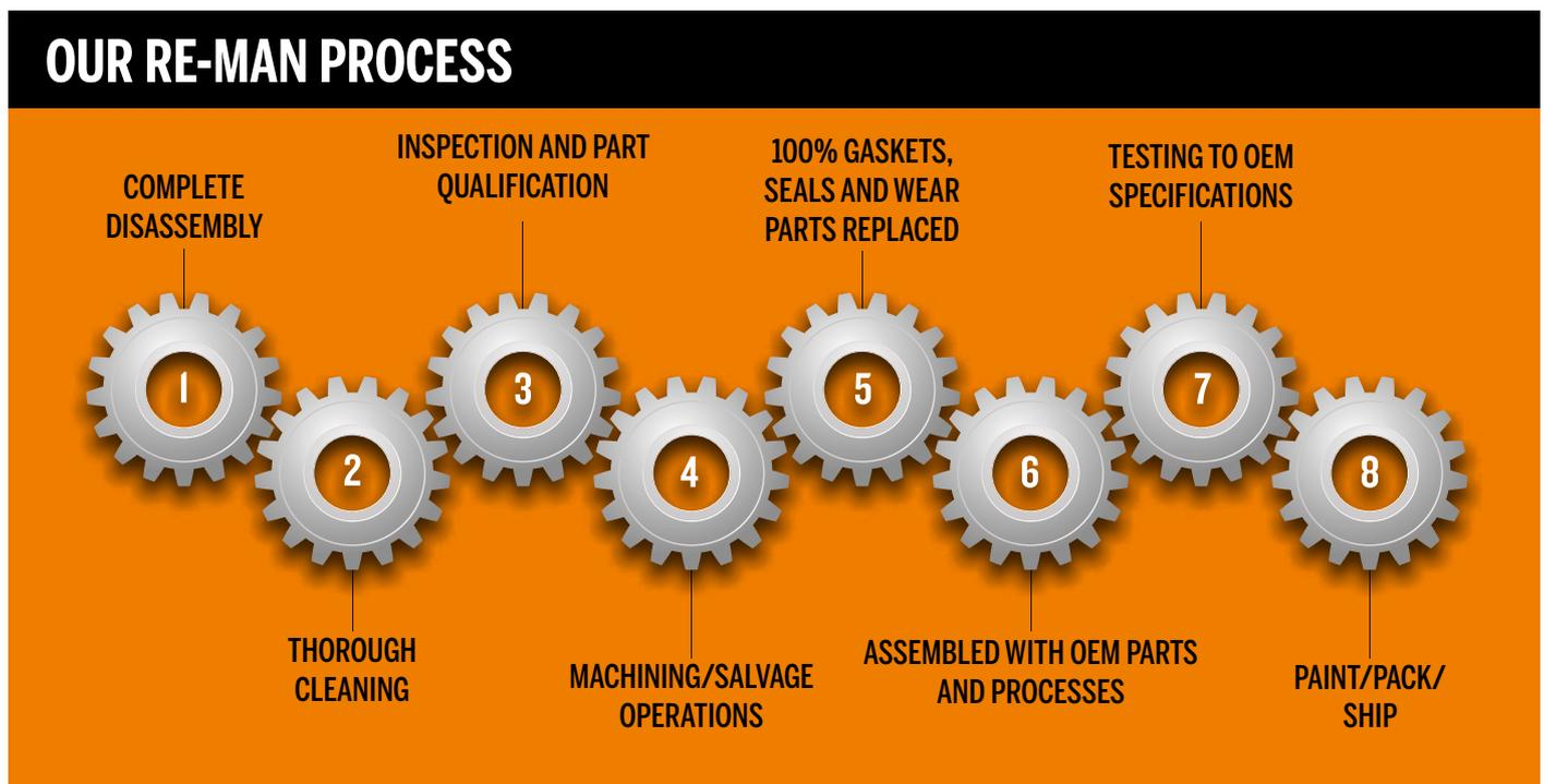
To make sure that our Re-man components live up to customer expectations, we leave nothing to chance. Each component is completely disassembled to allow a thorough inspection of the individual parts.
